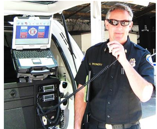
Multiple radios, including VHF High Band, are found in all Fire Service Battalion Chief units; this photo of Laguna Battalion One.
