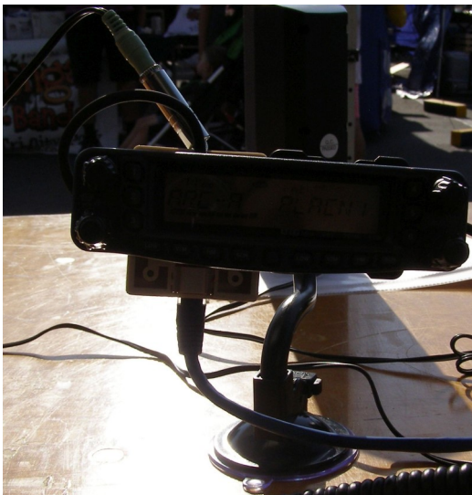
The radio's head on a gooseneck suction cup, set on a table outside of the MVC.
