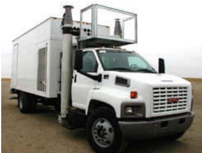
COLT (cellsite on light truck).
