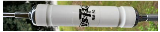
Hustler RM-60 60-meter resonator screws into the end of an MO-1 54-inch mast. A rod extends from the other end, which adjusts for resonance.
