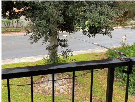
Hustler MO-1 mast with RM-60 60-meter resonator clamped horizontally to NH7WG's balcony railing, with a radial threaded in and out of the railing down to a ground wire. The railing itself could also be used as a counterpoise.
