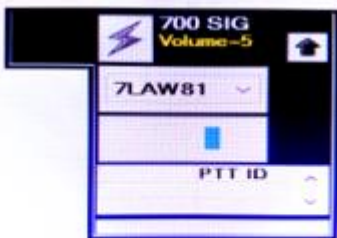
Screen shot of the Loma Ridge EOC public-safety radio console, inside the RACES radio room, showing one of the 700 MHz interoperable radio channels, 7LAW81, selected to the Signal Peak radio site.
