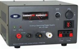
The MFJ-4275MV switching power supply delivers 75 A maximum and 70 A continuous. Input voltage is 110 Vac or 220 Vac. Load regulation is better than 1%, and ripple voltage is less than 12 mV peak-to-peak. MFJ claims that RF hash is eliminated. Front -panel output voltage is adjustable from 4.0 to 16 Vdc. Front-panel connectors include two pairs of Anderson Powerpoles, one pair of high-current five-way binding posts, a cigarette socket, and two pairs of quick connects. Weight is 10.5 pounds.
