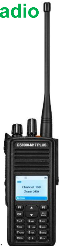
Connect Systems CS7000 M17 PLUS multiple-protocol UHF radio.
