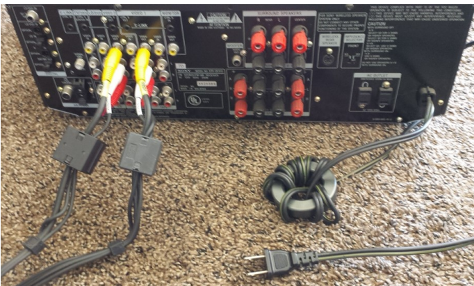
Palomar Engineers home theater system RFI kit consists of 17 filters for up to five A/V units plus I/O cables.
