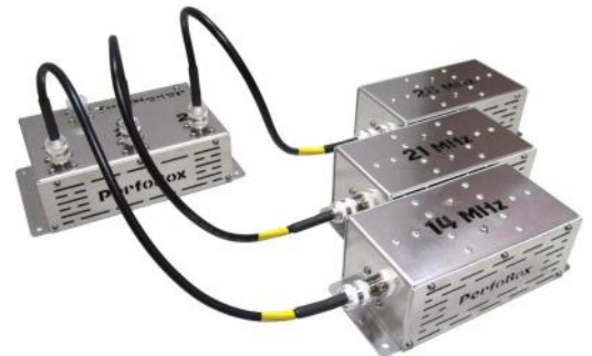
Triplexer with band-pass filters that enable three transceivers to operate on 20, 15, and 10 meters with only one multiband antenna.
