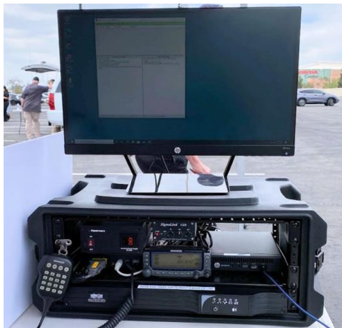
Transportable Winlink gateway KM6RTE-10 on 431.075 MHz at Radio Rodeo. The UPS is in the lowest section of the rack.
