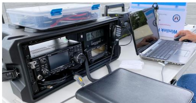
Portable Winlink Express client station at Radio Rodeo with radio equipment in transport case and laptop computer.
