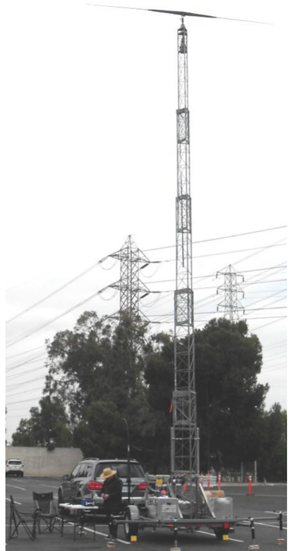
Trailer-mounted tower and military dipole were used by Gary Standard, K6GSX, and Peter Putnam, NI6E, on 40 meters at the Honda Center.
