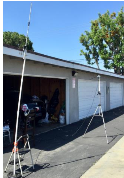
The antennas at the portable station of OCRACES Member Tony Scalpi, N2VAJ, included a 2-meter vertical (left) and a Hamstick dipole.
