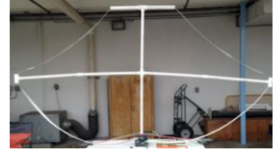
Tony's 40-m magnetic loop antenna.
