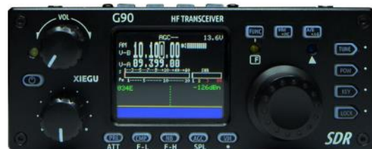
Xiegu's C90 front panel includes a \pm 24 kHz bandwidth spectrum display with waterfall.
