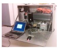
Open ComBox showing VHF/ UHF radio, TNC, laptop, and printer.
