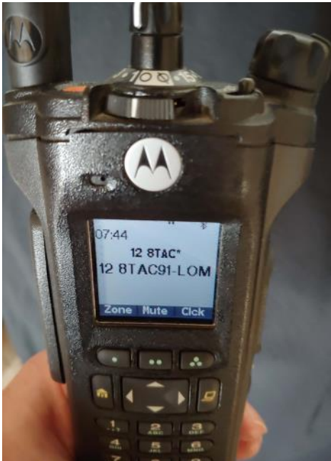
APX portable radio tuned to 8TAC91-LOM, a conventional repeater using an Orange County specific CTCSS. These channels appear in Zone 12 of all CCCS radios, shown by the leading 12 in the channel display.
