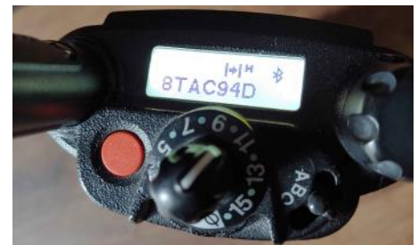
Top view of Motorola APX portable radio, which includes a small screen to display the radio channel name. Here, the radio is selected to 8TAC94-Direct.
