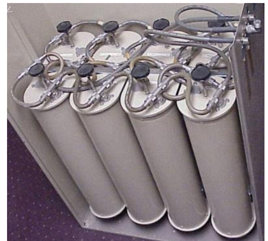
In this eight-cavity duplexer for a 2-meter repeater, four notch cavities are used for receive and four pass cavities for transmit.
