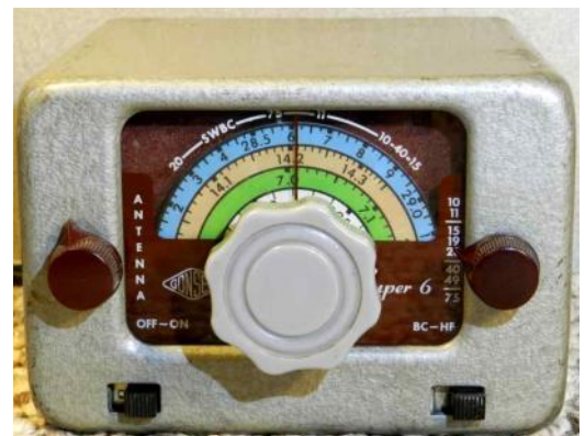
Gonset Super 6 converter allowed an automobile's broadcast radio to receive AM signals on the 80 through 10 meter ham bands.
