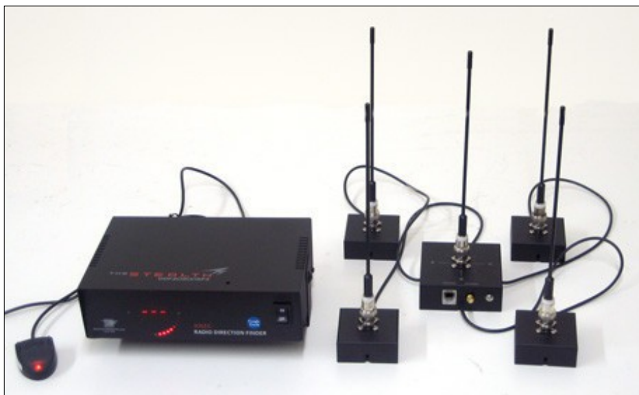
DDF2020T radio direction finder kit. Antennas are not included. GPS receiver is optional. User must provide VHF/UHF receiver and laptop or PC.
