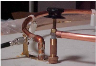
it would have looked like we installed the tail section of a Cessna 150 on the roof of the Van! The current model under consideration was found in the ARRL antenna handbook as a "DDRR" antenna. It looks like a 22 inch in diameter loop suspended 2 inches above the ground plane roof (see photos).
