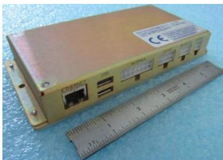
Doppler Systems DDF7001 DF processor can be used with a variety of receivers for either fixed or mobile operation. A provided Windows-based software suite enables the user to display lines of bearing on a map in real time. It is network compatible.
